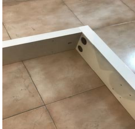
UNION BETWEEN SIDERAILS WITH INTERIOR FOOTBOARD
